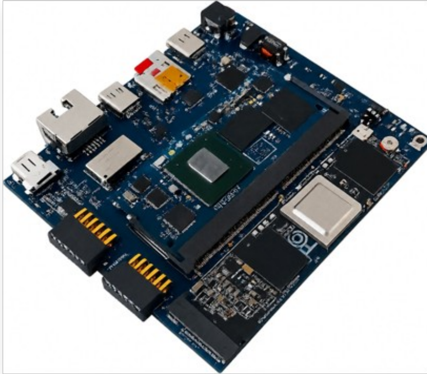
Figure 1 - The ZU-NEXUS-AI Kit with the ATLAS ZUS3 SOM installed in the SODIMM socket: RJ45, HDMI-size DisplayPort, USB and boot microSD on the left edge, PMOD headers on the front edge, M.2 slot area on the right.
